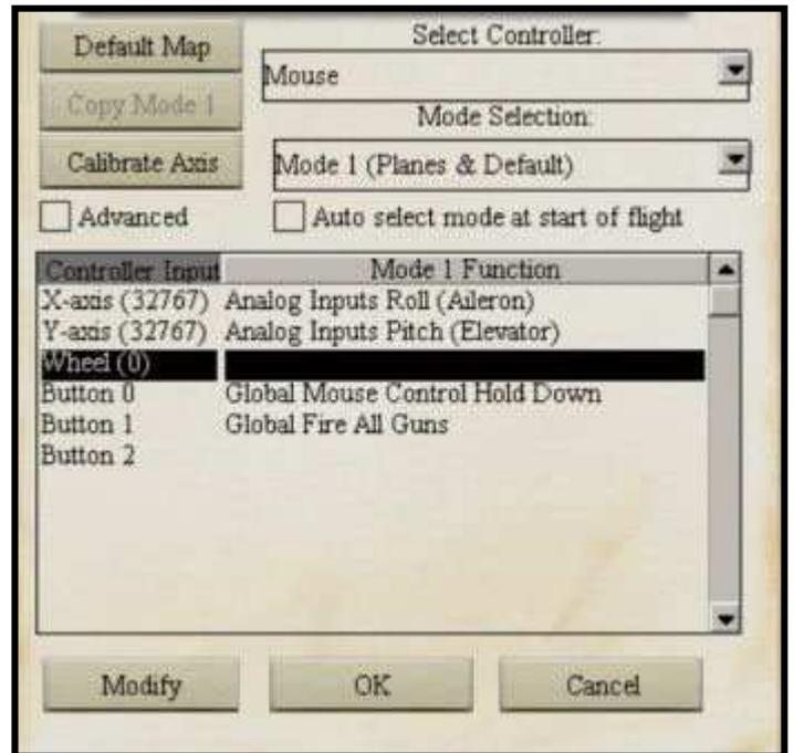
First we want to assign the throttle to the scroll of the mouse wheel.
